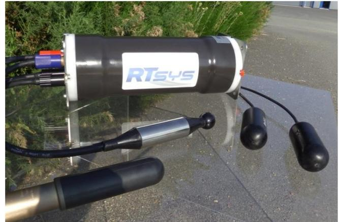
**EA-SDA** is a compact autonomous recorder that can simultaneously acquire the data of 4 wideband hydrophones. RTsys systems are thoroughly calibrated to be compatible with all international regulations.
